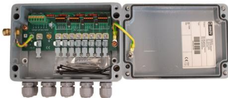
132690 DOL 199 Lightning protection
